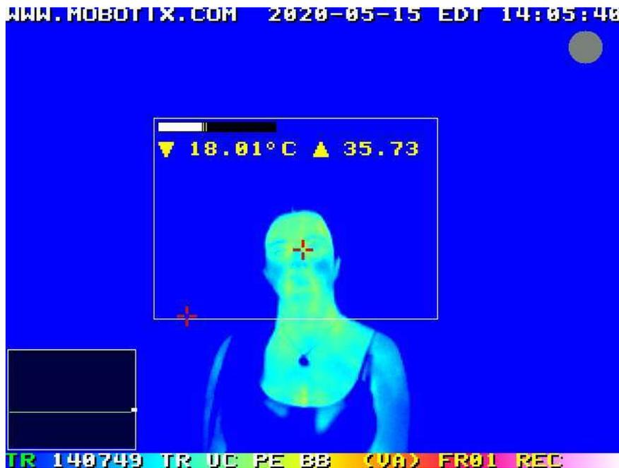
Note: Please note how the overall thermal signature is affected by the air being blown by the lens area
