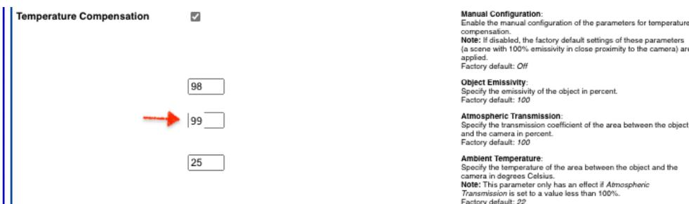
Always click [SET] to enable changes after changing the value. You can also adjust the Object emissivity if needed to 97, or to 99.
