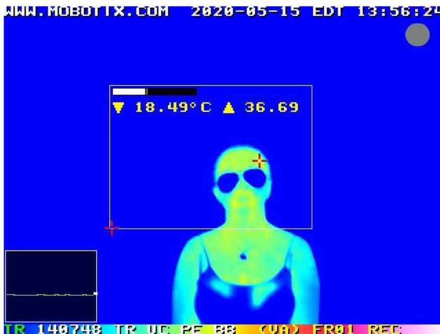
Note: A body temperature difference can be present if a person's face if measured in the forehead versus inner canthus (inner eye area), or versus any other spot in the face.
