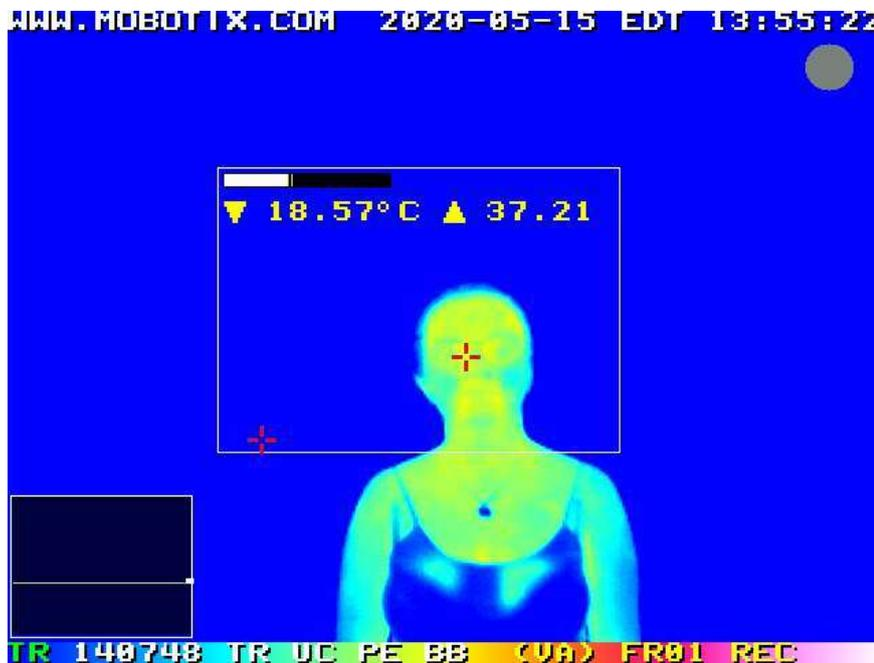
Note: The MOBOTIX Thermographic cameras TR will measure the hottest pixel in the area of measurement
