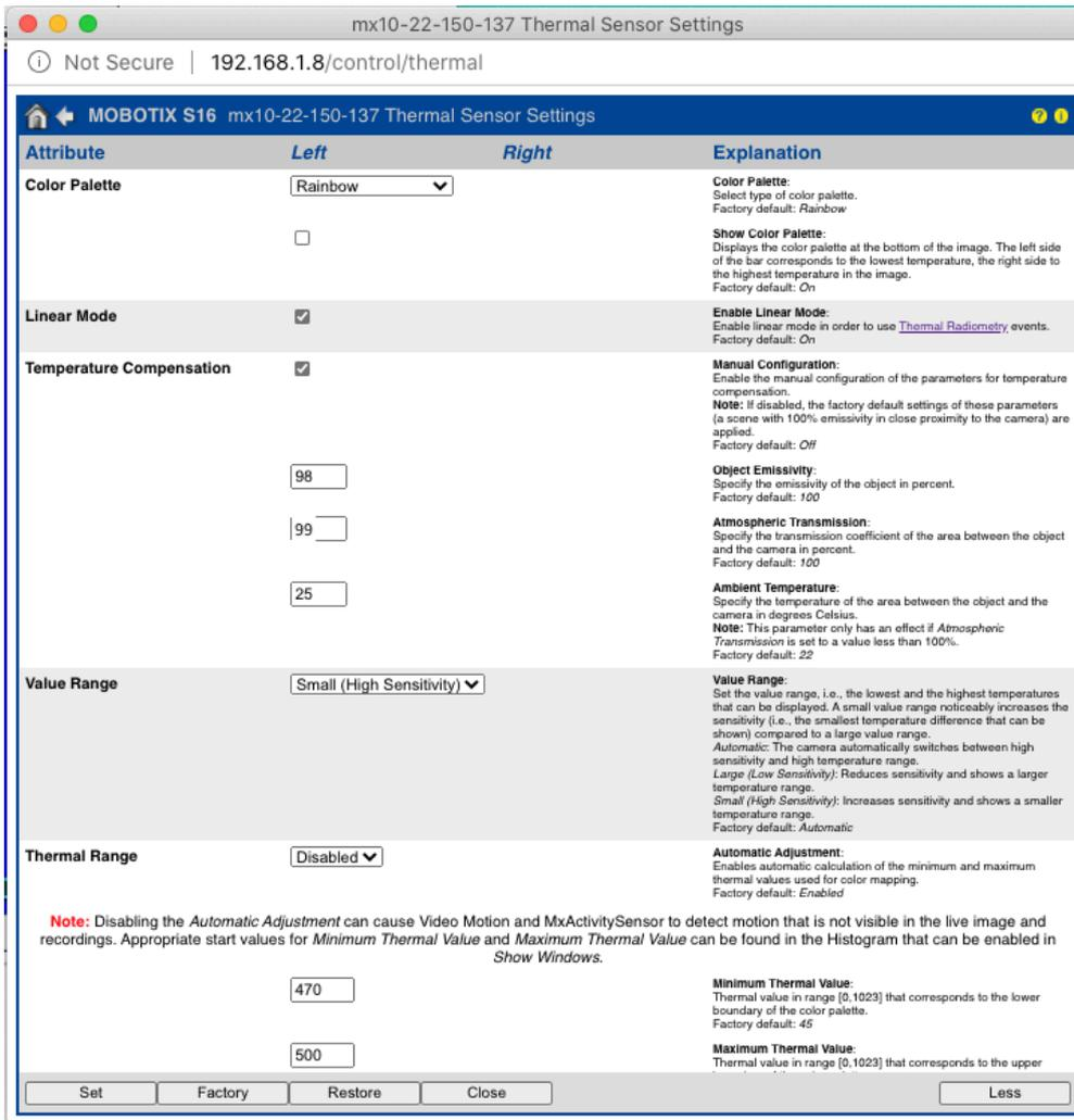
Adjust the Atmospheric transmission down from 99 in decrements of 5 points, 3 points, etc until you match  $\pm 0.3C$  to  $\pm 0.5C$  of the temperature measure by the clinical thermometer
